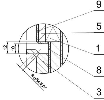
Fig.3b: Detail of conical head in regime "open"
