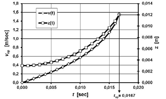
Fig.11: Dynamic characteristic for mode "opening"
