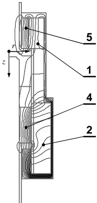
Fig. 8: Distribution of magnetic field lines in the regime "opening"
