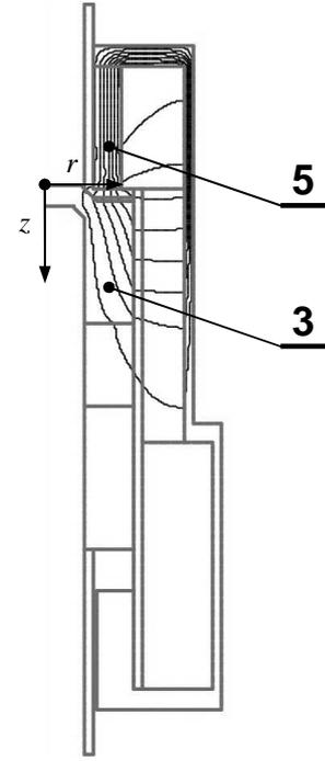
Fig.5: Distribution of magnetic field lines in the regime "closed"
