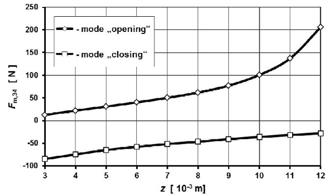
Fig. 9: Static characteristics for modes "opening" and "closing"
