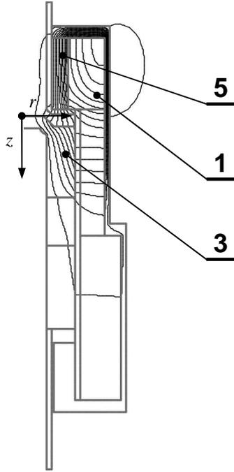
Fig. 7: Distribution of magnetic field lines in the regime "closing"
