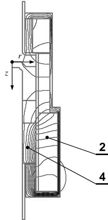
Fig.6: Distribution of magnetic field lines in the regime "open"
