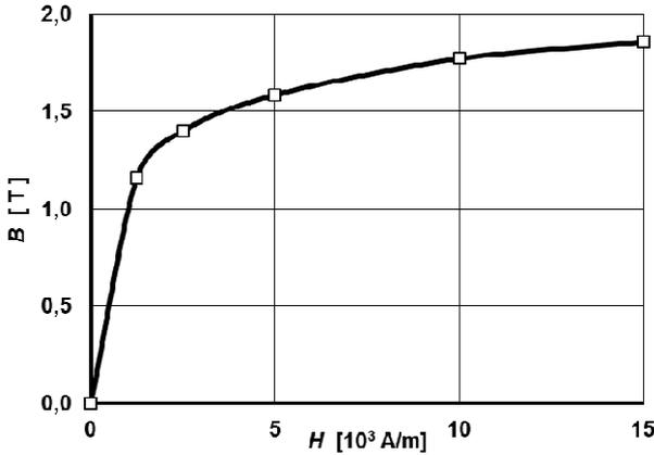
Fig.4: Nonlinear characteristic of steel ČSN 12 040
