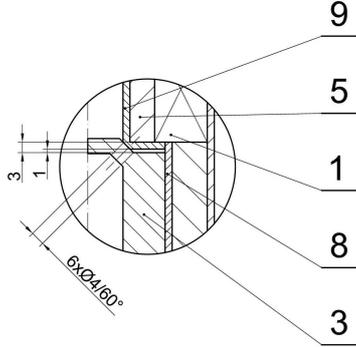
Fig.3a: Detail of conical head in regime "close"
